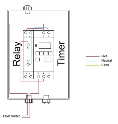
The control panel is supplied with wiring installed in the drawing shown above. The timer is always energised, and when programmed will output voltage via the float switch to the relay during the times set on the timer.
