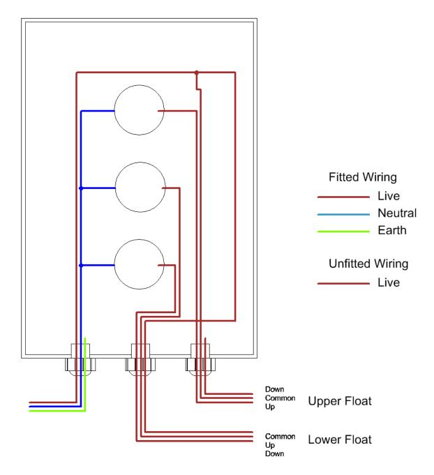
The lower float is wired with all 3 wires connected, the upper float uses only 2 wires to activate the green light. This achieves a sequence from full to empty of Green+Amber, Amber, Red.
