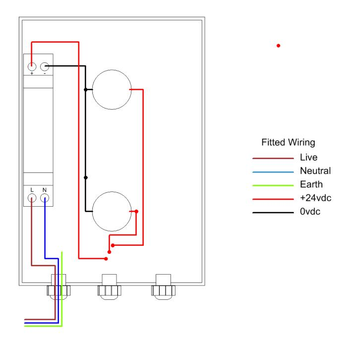
The control panel is supplied with wiring installed in the drawing shown above. The float or level switch needs to be fitted as shown in the next diagram.
