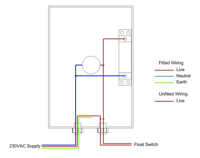
Note that both wires to the float switch or level switch are live.
