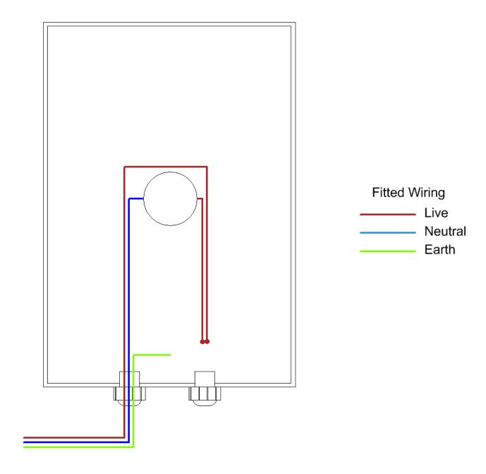
The control panel is supplied with wiring installed in the drawing shown above. The float or level switch needs to be fitted as shown in the next diagram.
