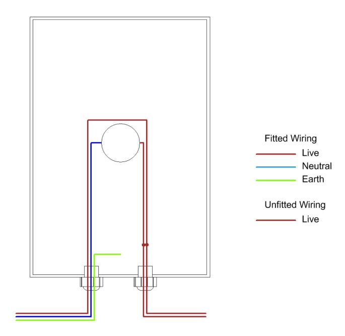
Note that both wires to the float switch or level switch are live.
