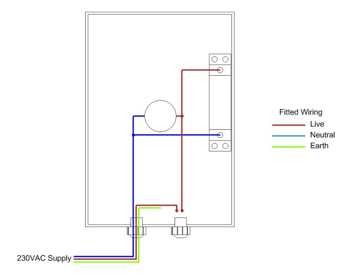
The control panel is supplied with wiring installed in the drawing shown above. The float or level switch needs to be fitted as shown in the next diagram.
