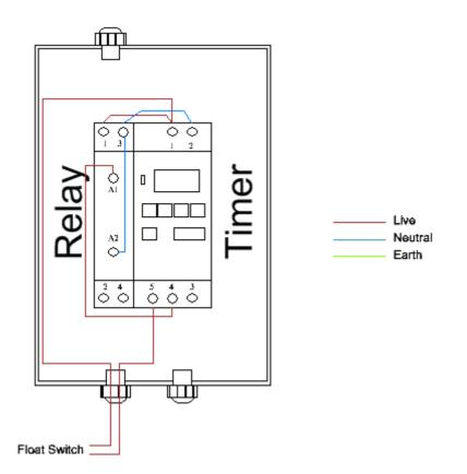
The control panel is supplied with wiring installed in the drawing shown above. The timer is always energised, and when programmed will output voltage via the float switch to the relay during the times set on the timer.
