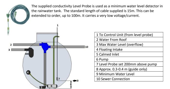
Fix the Level Probe in the tank so that it is suspended approximately 0.3 to 0.4 metres above the bottom, depending on the shape of the tank and position of pump inlet. It should be positioned to ensure there is no risk of cavitation or air entrainment to the pump inlet. If in doubt you MUST consult an approved and qualified plumber. The height of the Level Probe determines the minimum water level of the tank at which the pump will run.
