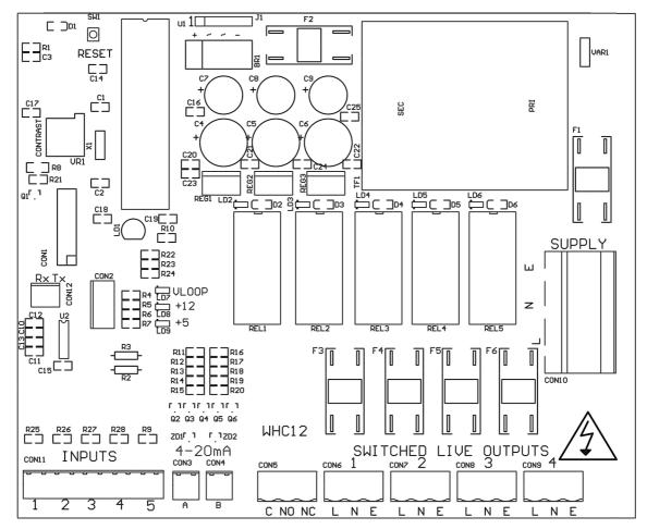
Each switched input is also designed to operate correctly with 3P Technik conductivity probes
