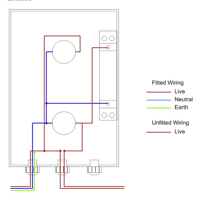
Note that both wires to the float switch or level switch are live.
