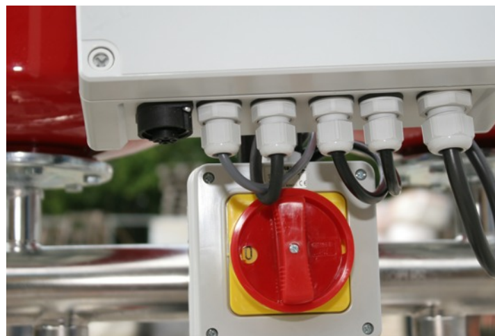
All electrics to IP65 ingress protection
